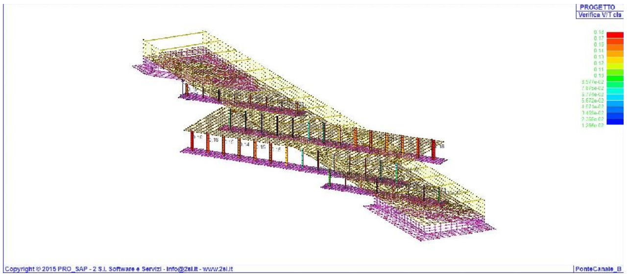
Pilastrini : Verifica V/T (lato cls)
